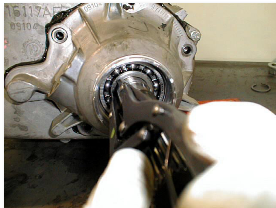
(Fig. 7) Rear I.D. Snap Ring Removal
