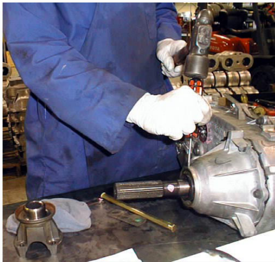
(Fig. 5) Rear Seal Removal
