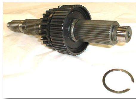
(Fig. 4A) (Large) Retaining Ring Installation
