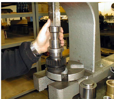
(Fig. 2A) Pull the Needle Bearings Out
