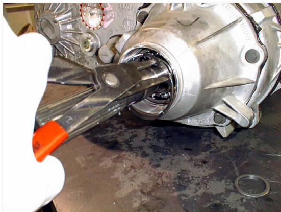
(Fig. 6) Rear O.D. Snap Ring Removal
