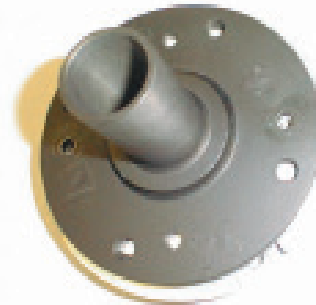
716067A retainer indexed over the stock GM retainer.
