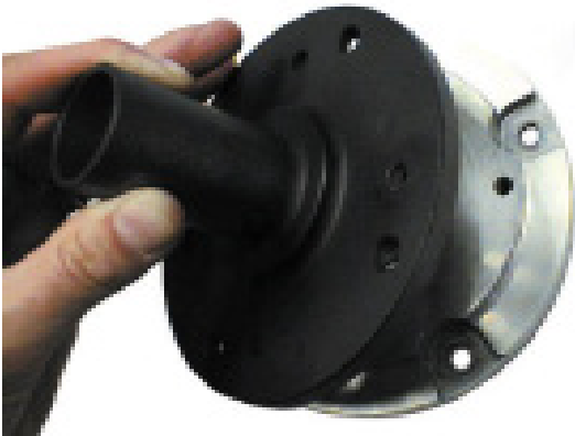
Line up holes of the modified retainer with the GM retainer holes.
