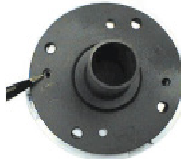
Make sure the modified retainer lines up with the two drilled & tapped holes on the GM retainer.
