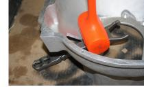
The new pivot ball needs to be installed into the bellhousing. Apply blue Loctite to the threads and torque to 40-45 ft-lbs. The clutch fork will need the spring clip installed; a pair of needle nose pliers works well. Once the spring clip is installed, apply grease to the spring and socket of the fork. \*Note: Clutch fork must be installed into the bellhousing before bolting to the engine.
