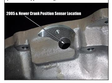
USE ORIGINAL DOWEL BOLTS FOR SENSOR, TO MOUNT TO THE NEW BELLHOUSING
