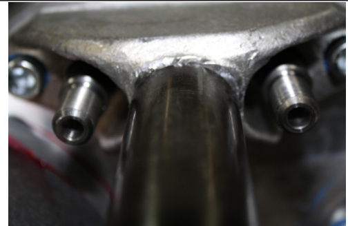
New shift rails with clearance holes drilled
