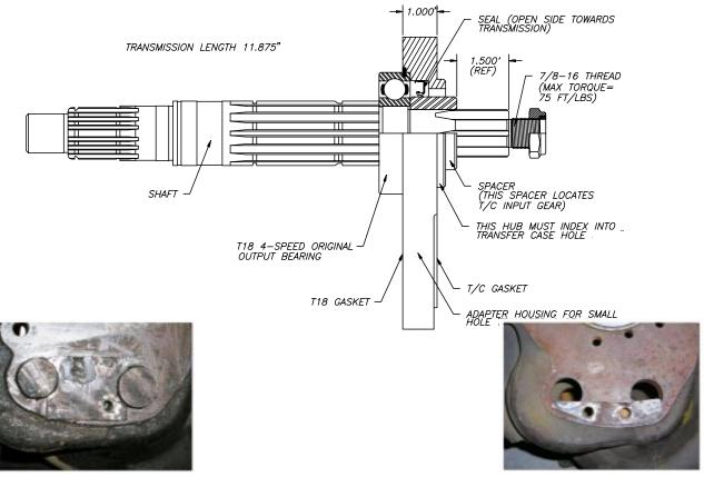
Some transmissions may require a modification to the cluster pin/reverse idler pin retaining bar. There are several different styles of this bar and a few will interfere with the mounting of our adapter plate to the transmission. Before final assembly, check the adapter plate for clearance and modify the retaining bar if necessary.
