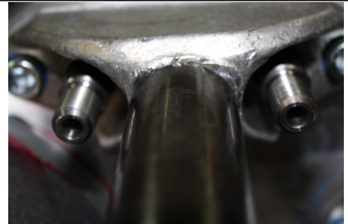
New shift rails with clearance holes drilled
