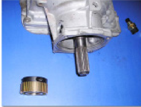
2. The clamp on reluctor gets installed onto the 700R output shaft and locked into position. If a 4L60E shaft is to be used, a different set collar is needed.
