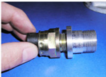
7. Remove the bushing after test fitting and then install the new reluctor sensor.
