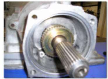
3. Reluctor ring installed
