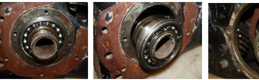
Remove the tailhousing bolts and front retainer bolts (if your transfer case has a front retainer). Shift the transfer case into 2WD high range and remove the tailhousing from the transfer case. Once the T/C output is removed, shift the T/C into low range which will release the slider. Remove the snap ring from the shaft to the bearing so the shaft and the bearing can be separated. This will allow the gear to drop downward and clear the shift fork.
