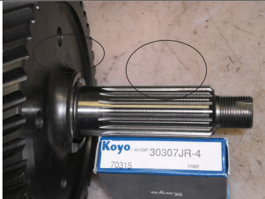
Lower two bosses that need to be modified for the cluster gear.
