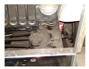
The 716838 is a cast steel plate that welds to the frame rail and can be used for Jeeps as well as Toyota L/C's. The tab sets on the frame rail and allow clearance for the bolts to mount to the factory steering box mounting holes. A clearance hole will need to be made for the steering shaft.
