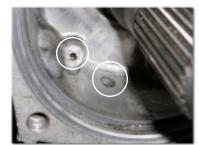
1/4" drill and work your way up until the 7/8" hole is obtained.
