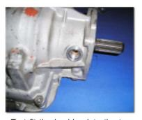
Test fit the bushing into the transmission housing. Make sure the bushing fits snug to the outside of the transmission. Note: You will have a small gap on the top and bottom side of this bushing, between it and the transmission.
