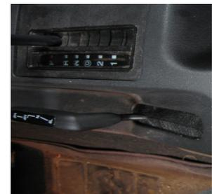
**NOTE: If the stock shifter bolts are missing or have been discarded. Replace with five 10-32" X .625" bolts or screws and washers.**
