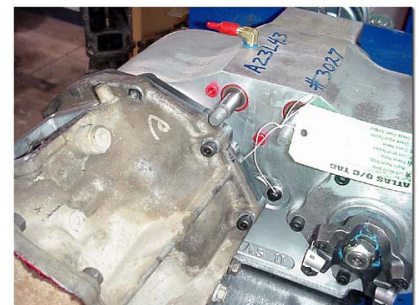
Left hand transfer case. The shift rod requires a extension rod to provide additional clearance. The Atlas also requires a speedometer housing for the transfer case.
