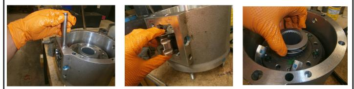
Remove the shift rail so that the shifter fork can be removed. Once the fork is removed, the drive hub can be pulled from the unit.
