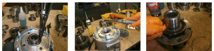
Flip the unit over to gain access to the snap ring on the front input. The seal will need to be removed from the casting. The planetary assembly and the input are now ready to be removed from the housing. The bearing is a light press fit to the input and the input may need to be tapped slightly to be removed.
