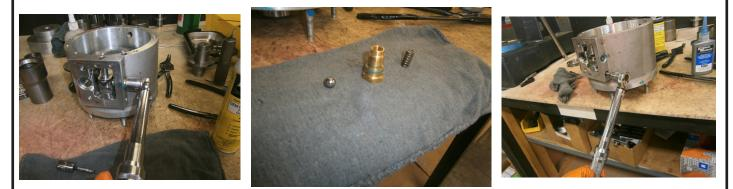
Remove the shifter detent spring and ball. Remove the set screw that holds the shift rail in the case.
