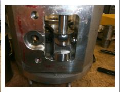
Remove the top shifter from the planetary housing.
