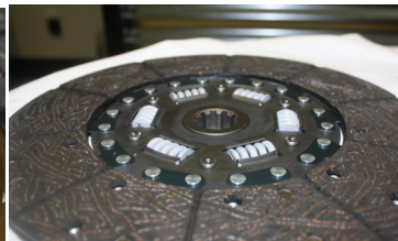
Clutch hub clearance on the flywheel P/N712546G vs 383735
