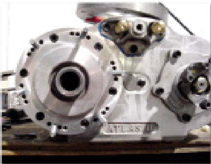
The photo (left) shows the rotation we used to obtain the proper shifter clearance.
