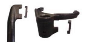
Install the O-ring on the front of the 51-9111 casting. Install the 4 stud bolts and locktite them into the crawler adapter plate. Then install the 51-9111 casting and secure it to the crawler adapter.
