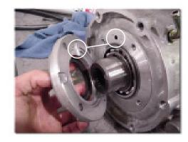
During reassembly, make sure the oil return hole matches the front retainer hole.
