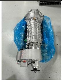
10R140 connected to the Atlas. the lower photo shows the gap from the splines of the transmission to the Atlas input. AS-8610 will allow the two to mate correctly
