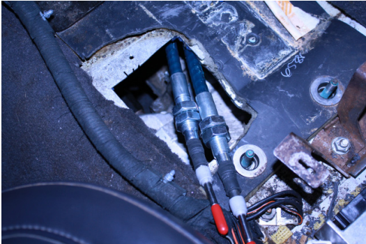
Cables connected to the new box and then test fitted and shifted to make sure the shift throw clears the slot.
