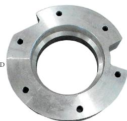
In order to provide clearance for the shift mechanism on the NP205 T/C, you must make a small relief area in the original 4WD tailhousing. If you do not have a milling machine, then you can remove this excess material by using a drill press and drilling numerous holes. The photos on this page illustrate the modifications required.
