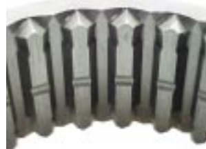
This photo shows the taper of the splines on the shifter slider.
