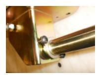
After attachment to cable shifter housing, cycle though all shift points and adjust if shift lever hits the inside of the shifter housing. Install boot retaining ring into supplied shifter boot. Attach shifter housing to vehicle floor using supplied 1/4" fasteners. Attach shifter boot to shifter housing using (4) supplied self tapping screws. Install shift knob jam nut and shift knob.
