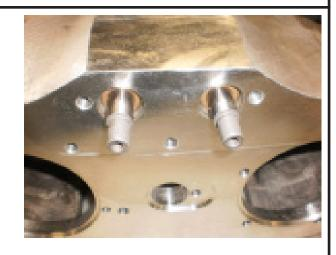
torqued to 35 ft.-lbs. NOTE: We manufacture two of these cable mounts, one for a left drop case and one for a right drop case. The mount will only fit the case drop it was designed for.
