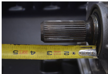
Stock 4WD output shaft with 3.375" of spline. This spline should be recessed from the casting face .325" once the casting is installed.
