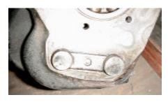
Some Jeep T18 transmissions will also require the idler shaft strap to be bolted or secured to the case. The easiest way is to drill and tap a hole in the center of the strap as shown above. If your T18 has the strap bolted to the case, you will not have to worry about this procedure.
