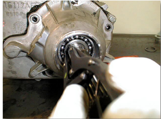
(Fig. 7) Rear I.D. Snap Ring Removal
