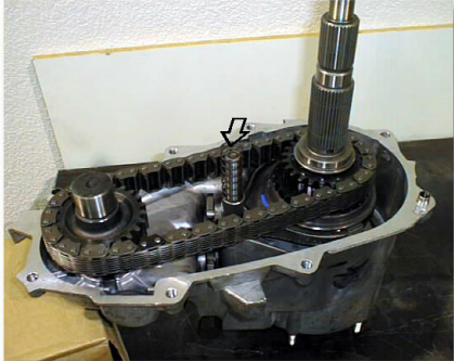
(Fig. 5A) New Main Output Shaft Assembly
