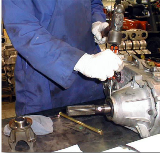
(Fig. 5) Rear Seal Removal
