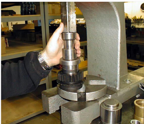
(Fig. 2A) Pull the Needle Bearings Out
