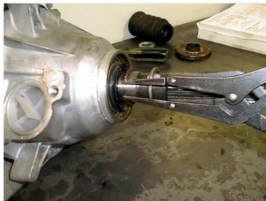
(Fig. 4) Stop Spacer & Snap Ring Removal
