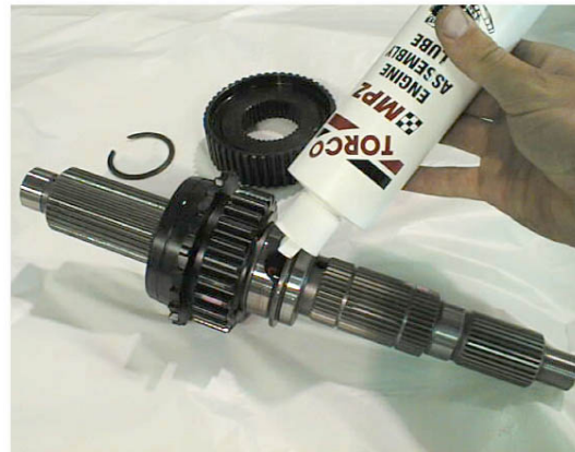
(Fig. 3A) New Main Output Shaft Assembly
