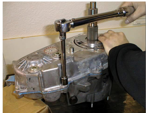
(Fig. 8A) Case Halves Assembled
