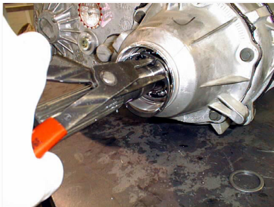
(Fig. 6) Rear O.D. Snap Ring Removal
