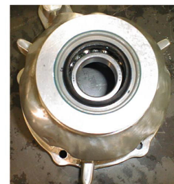
(Fig. 11A) Seal Installed
