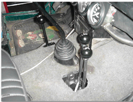
Twin sticks through modified hole in floor.
