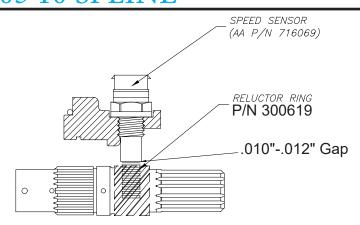
**Sensor note:** The sensor in this kit was changed in October 2005. This sensor will match up with the GM pigtail P/N 12162193 or Carquest P/N TX3A. The old sensor used in earlier kits matches up to GM pigtail P/N 12085498.
