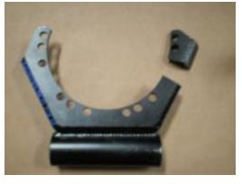
The mount needs to be cut to provide clearance for the transfercase shifter linkage bracket.
