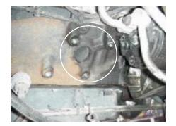
The stock passenger side mount must be removed. The passengers side LT1 mount used an inverted triangular mount; however, this block also had the standard Chevy mount configuration. The top front hole of the standard mount on this block was used as a support for the air conditioning pump (shown center photo).
