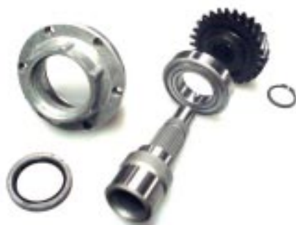
AA shaft & bearing with stock parts
