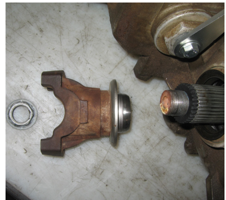
Figure 31: Proper Yoke Installation Order
