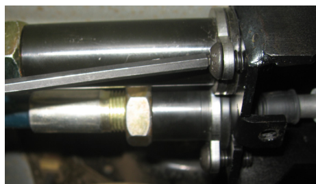
Figure 22: Tighten Retaining Clip
