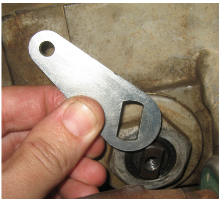
Figure 30: New Transfer Case Shift Lever Orientation
