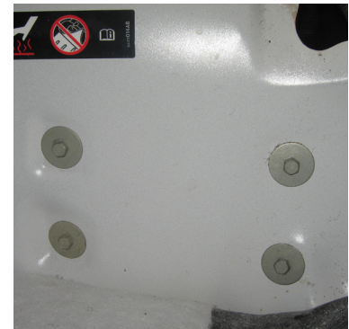
Figure 12: Shifter Pivot Assembly Bolts
