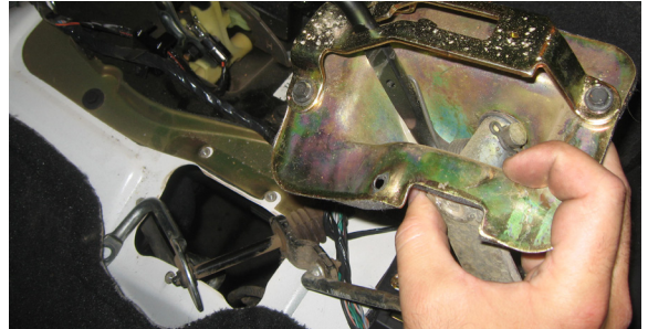
Figure 13: Remove Shifter Linkage
