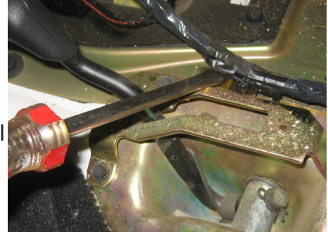
Figure 11: Remove Wire Loom Connector Clip
