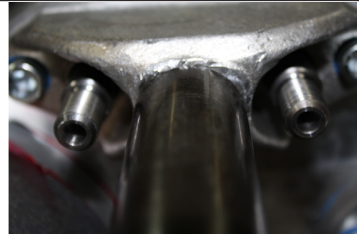
New shift rails with clearance holes drilled
