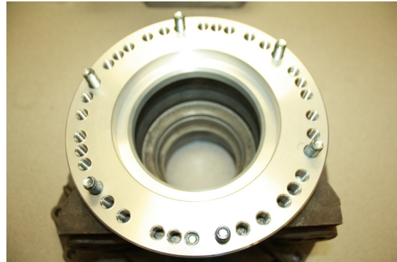
Install the 6- SHCS bolts through the two adapters and secure them to the NP205. Photo shown is the Allison tailhousing with the 51-8603 installed.
