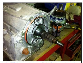
On 2WD transmissions the holes located at 12 and 6 o'clock need to be plugged with factory soft plugs. The output shaft needs to have a seal installed. You also need to check the NP205 input length so that it does bottom out on the 2WD output shaft o-ring. If it does hit the o-ring, you will need to trim the input gear to fit.
