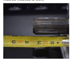
This casting is designed for the stock 4WD output shaft. The 6L80 shafts are 32 spline.
