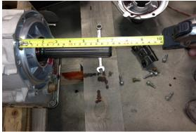
6.75" stickout on a 2WD transmission. the shaft will need to be cut or shortend to 3.30" long. the casting is installed.
