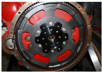
Once the crank is exposed, install the new flex plate onto the block as shown. Use the factory bolts to secure the flex plate to the crank and torque to 55 ft.lbs. The crank adapter will need to be mated to the flex plate as shown and then secured using the 12MM bolts and flat washers, torque bolts to 55ft.lbs. If your block has the factory dowel pins located at 12 & 6 o'clock, they will need to be removed.
