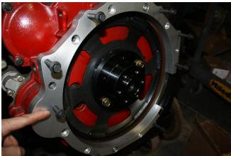
The bolts that mount the GM transmission to the new adapter plate are all 40MM long accept one that is 30MM. That bolt must be installed in the location shown and torqued to 30 ft.lbs.
