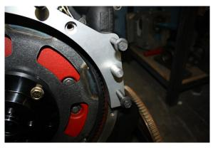
The GM dowels must be installed before installing any GM transmission. These can be installed before starting the installation process or tapped in place once the adapter is installed to the Cummins engine.
