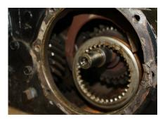
Remove the tailhousing bolts and front retainer bolts (if your transfer case has a front retainer). Shift the transfer case into 2WD high range and remove the tailhousing from the transfer case. Once the T/C output is removed, shift the T/C into low range which will release the slider. Remove the snap ring from the shaft to the bearing so the shaft and the bearing can be separated. This will allow the gear to drop downward and clear the shift fork.
