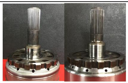
Note: 6L90 4WD transmission output shafts. We have seen two different lengths of outputs. One is simular to the 6L80 4WD and the other is longer. The longer shaft is approxamately 5" +/- stickout. Trimming this shaft will not allow enough splines to fit the transfer case. A 3/4" spacer (P/N AS-8603) will be needed and you will still need to modify the shaft length.
