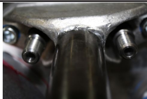
New shift rails with clearance holes drilled
