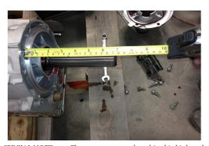
6.75" stickout on a 2WD transmission, the shaft will need to be cut or shortend to 4.00 cut off.
