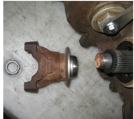
Figure 31: Proper Yoke Installation Order
