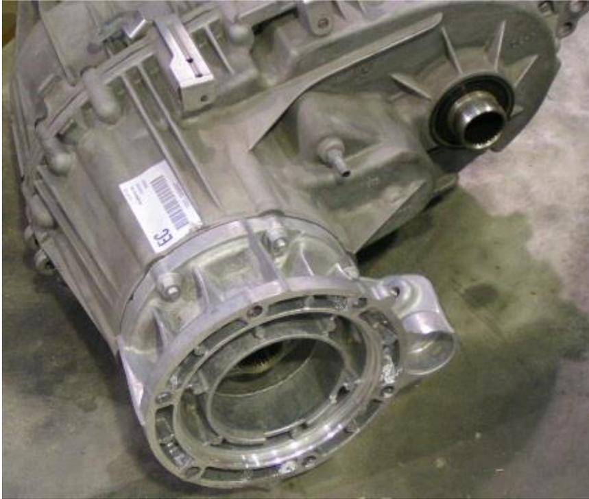
2. Measure 95mm to 97mm from the rear face of the transmission and mark the output shaft. **Note:** The 4wd transmission output shaft may not need to be cut down. See photo and diagram below.
