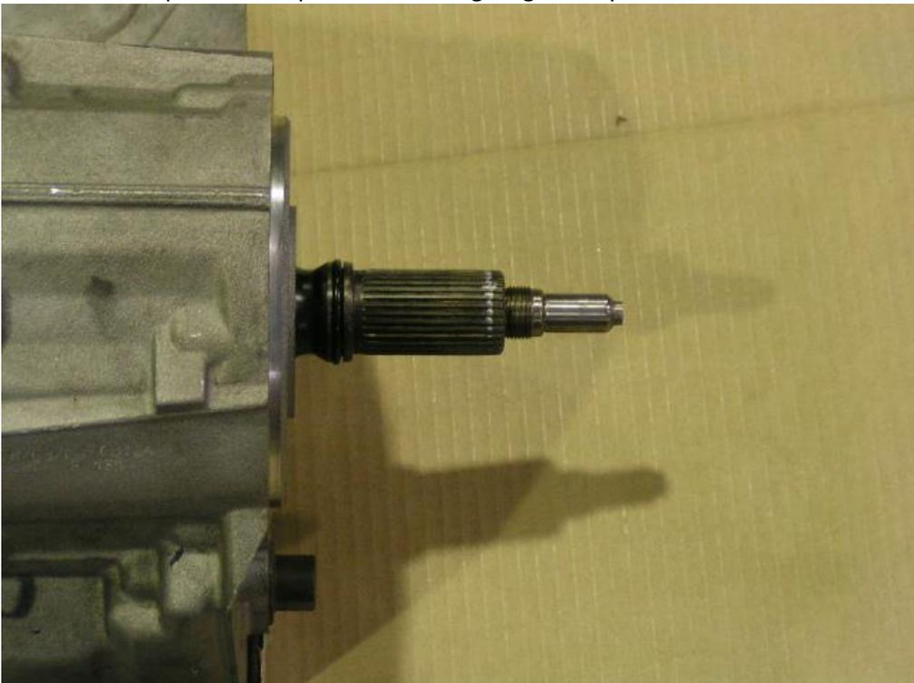
4. Check to make sure the coupler shaft fits over the previously cut and chamfered output shaft
