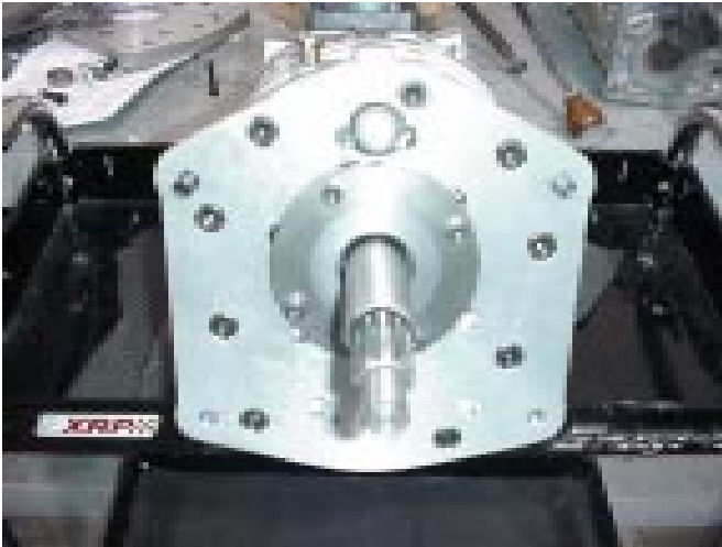
Adapter plate installed on the NV3550
