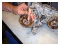
43. Reinstall the steel ball in the bottom of the case followed by the spring and the detent plug.
