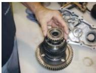
28. The input shaft/gear will now need the bearings removed and installed on the new shaft/gear. A press is usually needed to remove and install the bearings.
