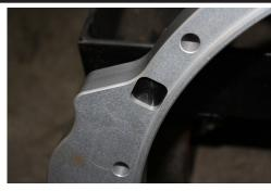
The new square headed dowel bolts need to be installed into the new adapter. the dowel portion of the bolt is a light press fit into the adapter.
