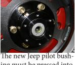
The new Jeep pilot bushing must be pressed into the crank adapter. This is a light press fit and has a machined pilot step for an easy install.
