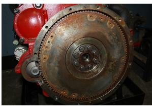
The Cummins block should have a factory flywheel or at least the factory crank bolts. The flywheel needs to be removed and the bolts retained for the new flex plate. The stock flywheel if equipped just needs a light tap on the bottom edge to remove it from the crank. The flywheel is not going to be reused.
