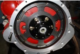
Install the SHCS bolts to the Cummins engine and torque to 30 ft.lbs
