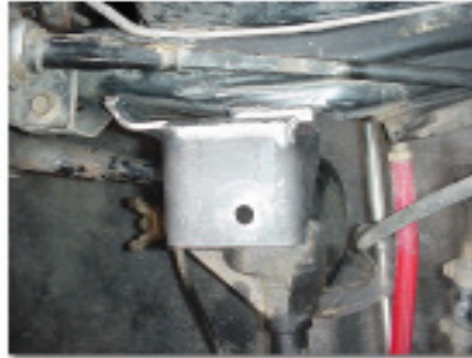
Driver's side frame mounts welded into position
