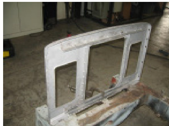
Completed modified radiator support
