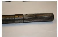
Trim shaft by measuring the 700R stock shaft stick out from the square bolt pattern on the transmission. Take that measurement plus the 1.800" on the new spacer adapter. By adding the 700R and the adapter measurements together, you can now measure from the back of the TH350 with this new amount and cut the output shaft to match the 700R stick out. The total amount that should be cut from the shaft should be no more than 1.50".
