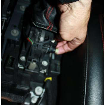
Remove the stock transfer case shifter. The parking brake will also need to be removed to access the floorboard mount that the cable runs through. The cable will need to be cut and pulled out of the rubber grommet.
