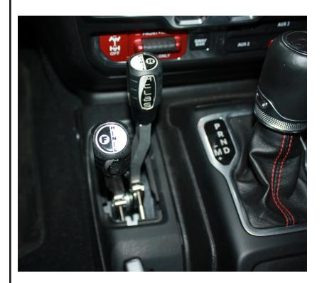
Install the shifter knobs and apply the shift stickers.
