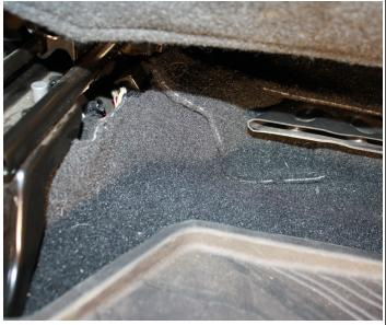
Remove the console. There are 4 10MM bolts, two in the front and two in the rear that the seats need to be slid forward to access. Also under the passenger seat there are 3 leads that need to be unplugged to allow the console to be removed.
