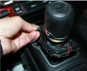
The transmission shifter needs to be placed in neutral and the boot ring needs to be pulled up out of the console. You can pull the boot up over the knob to access the bolt to remove the knob.
