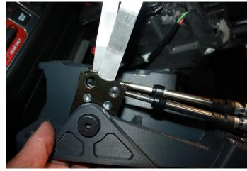
Once cable are secured the base can be installed into the console (Jeep tub) with the factory bolts.
