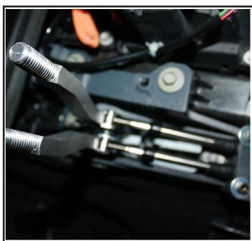
Once all connected, test shift and check to make sure you have clearance of the handles to the dash. If you have hooked the rear cable to the handle closest to the transmission shifter, 2WD high should be forward and the handle closet to the driver should be slightly angled back. Photo shown below.
