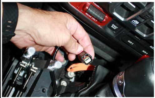
Once shifting if confirmed, install the console and make sure the auto transmission indicator light is re-connected and well as the plugs under the passengers seat.
