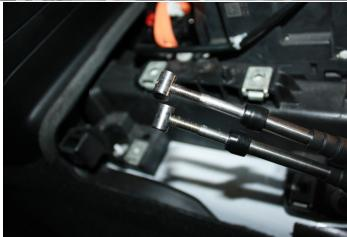
Install the cable connector ends so that the threads are flush.
