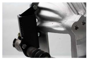
The new push rod has a ball end fitting that can be used up to the GM fork. To use the wedge connection, remove the ball fitting, thread on the new nut and install the wedge.
