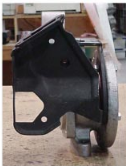
Jeep# 53005371 - This bracket is normally used with AX15 transmissions. This bracket mounts below the new linkage bracket.
